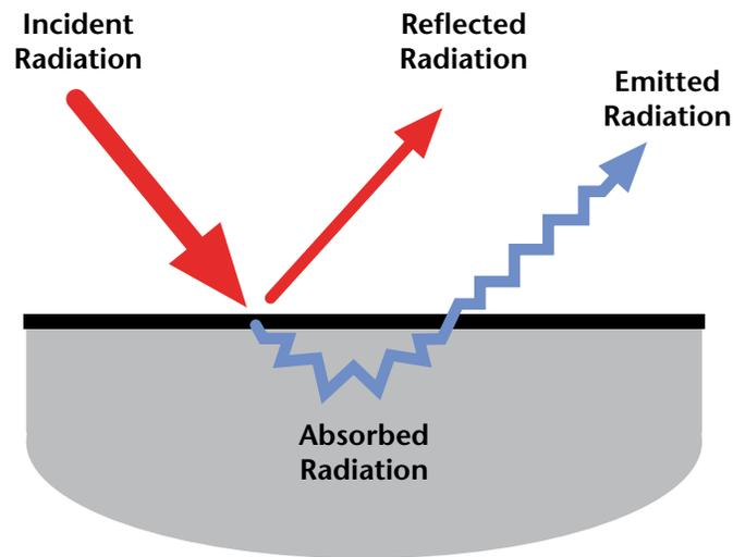
*For any particular wavelength of radiation striking an opaque material, the sum of radiation that is reflected and that absorbed must equal the incident radiation. The radiation emitted and the radiation absorbed must equal each other at steady state.*
